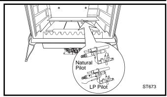
Fig. 30 Pilot assembly location.
